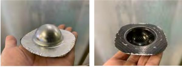
Fig. 12 Hemispherical press-formed product made of aluminum and CFRTP.
